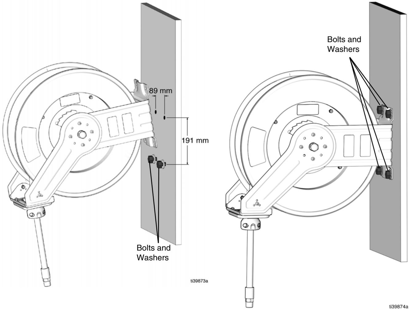
**FIG. 8: Typical Installation**
