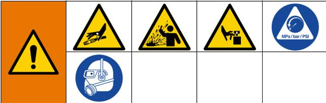
This equipment stays pressurized until pressure is manually relieved. To help prevent serious injury from pressurized fluid, such as skin injection, splashing fluid and moving parts, follow the Pressure Relief Procedure when you stop dispensing and before cleaning, checking, or servicing the equipment.
